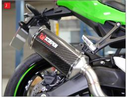
I) Place the plain clamp over the Scorpion connecting pipe then slide the pipe onto the original exhaust.
